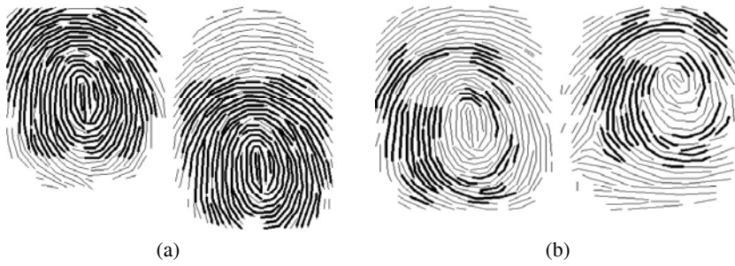
Fig. 1. (a) Match result for fingerprints from same finger; (b) Match result for fingerprints from different fingers. Thick lines represent matched ridges and thin lines represent unmatched ridges
